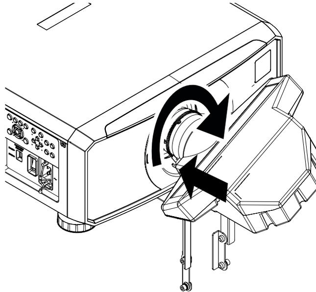
6. Attach the arms to the adapter bracket using the provided screws. Do not tighten the screws yet.
