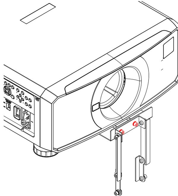
4. Make sure the adapter bracket is attached to the bottom of the lens.
