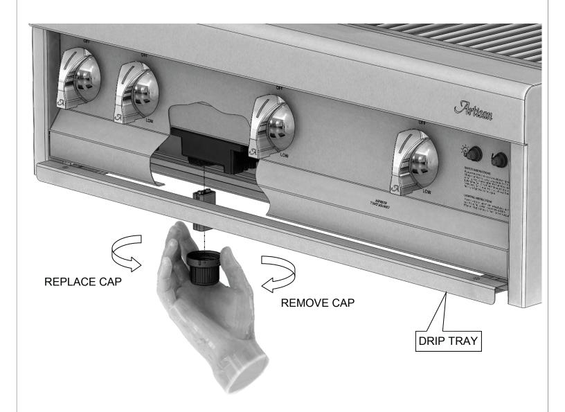
To insert or replace the battery which powers the igniters:
