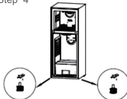
Unscrew and remove the two adjustable legs. Unscrew and remove the bottom hinge. Reserve the screws. Attach bottom hinge with the reserved screws.
