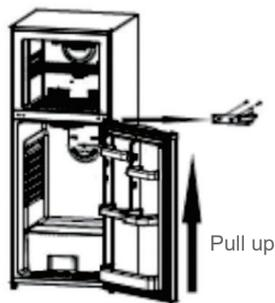
Unscrew and remove the middle hinge. Reserve the screws. Lift the refrigerator door up and away from the appliance.
