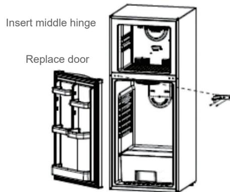
Place the refrigerator door on the bottom hinge. Ensure the door is aligned horizontally and vertically. Attach middle hinge to top (left) of refrigerator door, align with holes and affix to middle beam with reserved screws.
