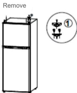
Remove top hinge cover. Unscrew and remove the hinge piece. Reserve the screws.
