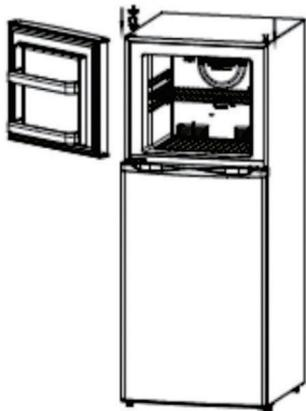
Place the freezer door on the middle hinge. Ensure that the door is aligned horizontally and vertically, and that the gasket seals on all sides before attaching the top hinge. Re-attach the top hinge with screws and place hinge cover over top.
