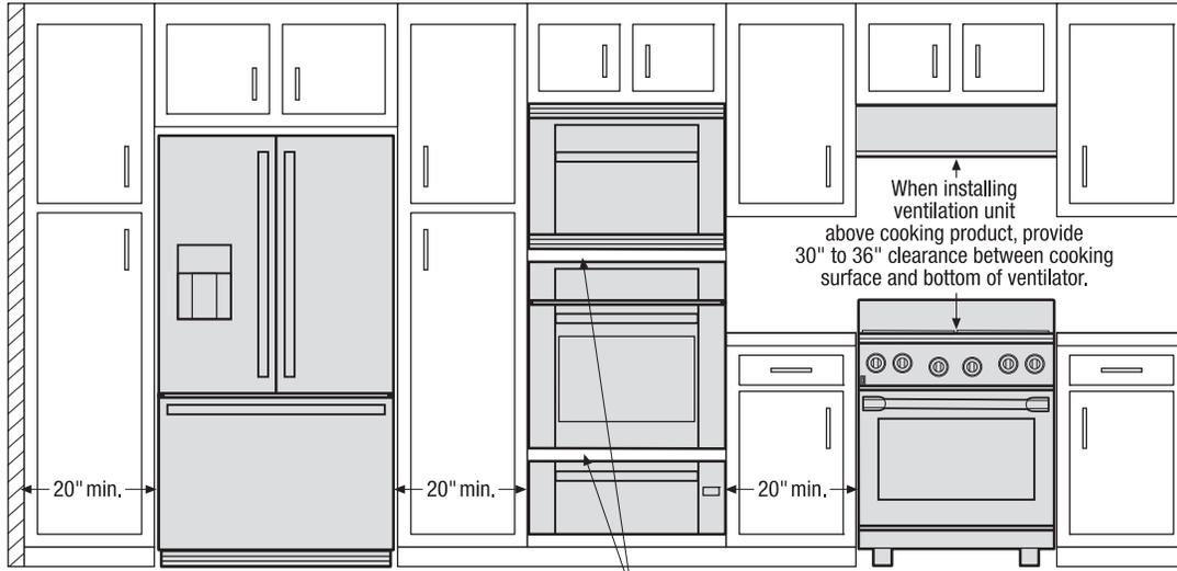
When installing appliances adjacent to each other, 20" minimum distance between each appliance required.
