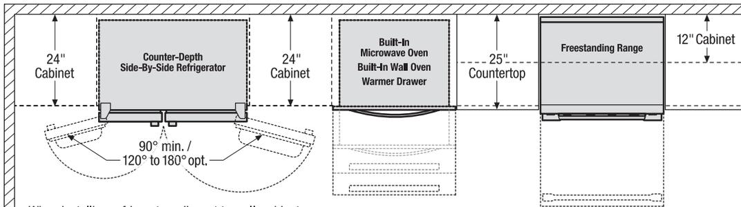
When installing refrigerator adjacent to wall, cabinet or another appliance that extends beyond front edge of unit, 20" minimum clearance recommended to allow for optimum 120° to 180° door swing, providing complete drawer/crisper access and removal.
