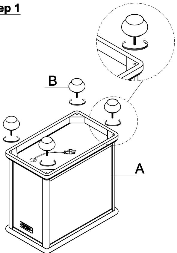
PLEASE DO NOT TIGHTEN THE BOLTS UNTIL ALL THE PARTS ARE IN POSITION
