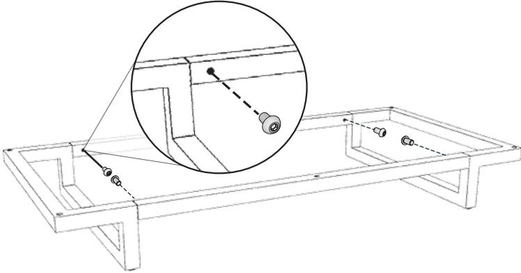
**B.** Attach tube base to your cabinet using connector bolt.
