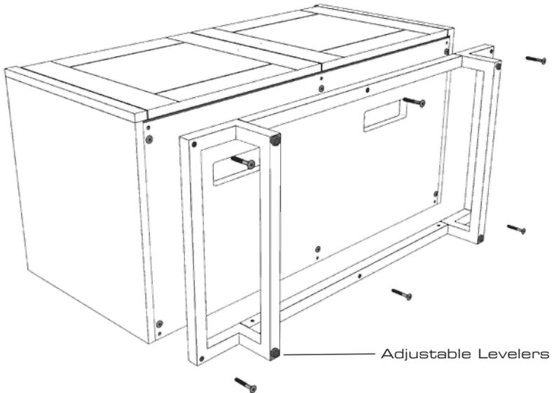
**C.** Secure tube base with washers and screws.
