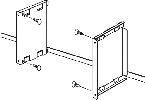
3. Secure upper bracket (with foam gasket) to the air diverters using the two (2) supplied push pins.
