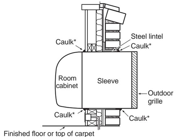
**NOTE: \*It is critical to caulk around the perimeter of the wall sleeve on all four sides on the outside and roomside where it joins the building to prevent air and water infiltration.**
