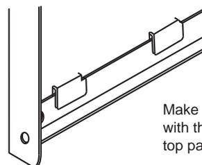
Make sure the panel engages with the tab on the bottom and top panels correctly
