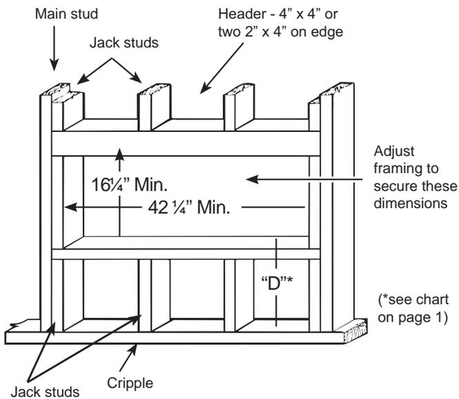
**NOTE:** Use lintel to support brick, block, etc., above the air conditioner sleeve. (If directly under a window sill, the use of a lintel may not be necessary.)
