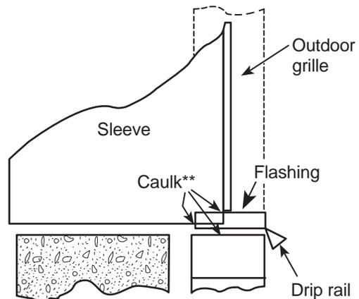
**NOTE: \*\*It is critical to caulk around the perimeter of the flashing and drip rail where it joins the building and sleeve to prevent air and water infiltration.**
