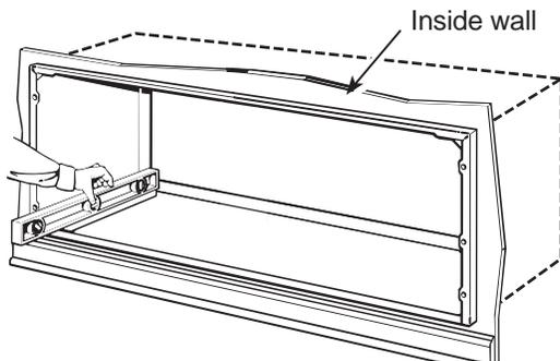
2. Firmly secure the sleeve to the wall structure. Do not drill any holes in the bottom of the sleeve.
