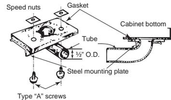
2. With an "External Drain" (which may be connected to a field-supplied drain line), condensate water can be drained away from the unit and building.
