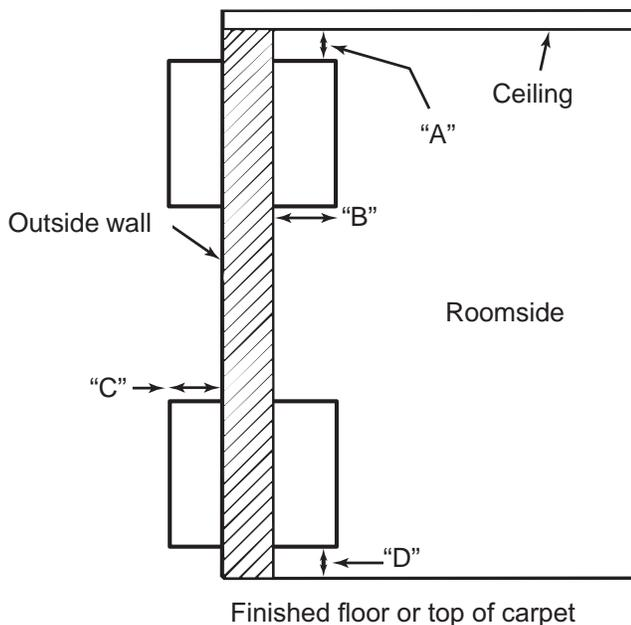
**NOTE:** Care should be taken in location of electrical supply entry in relationship to wall sleeve to ensure access to power once the unit is installed.
