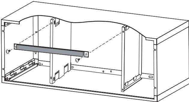
4. (If required) Locate weather barrier and attach to the rear of the assembled sleeve with four (4) supplied push pins.
