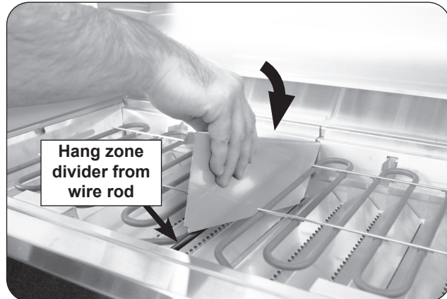
Fig. 28-3 Install zone divider
