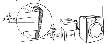
Minimum capacity: 20 gal. (76 L). Top of laundry tub must be at least 30" (762 mm) above oor; install no higher than 96" (2.44 m) from bottom of washer.
