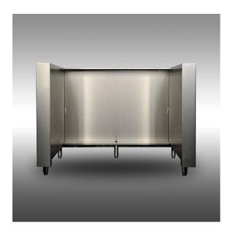
Insulating grill surround for use with K750GB built-in Gaucho grills. Adds 8-inches to the width of the grill. Do not use with combustible cabinets unless there is a minimum clearance of 36-inches between grill and combustible materials.
