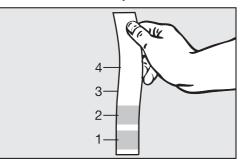
Dip the test strip in the water for approx. 1 second. Shake excess water off the test strip.
