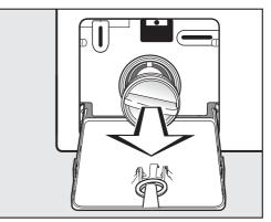
Remove the drain filter completely.
