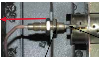
Diagram 2 Remove front nut
