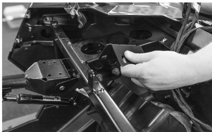
Slide the bracket between the nuts and the column support. Do not tighten yet.
