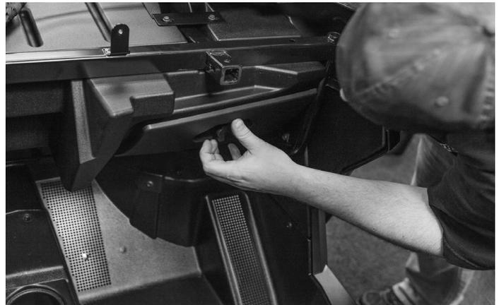
NOTE: The glove box latch mount that is pre installed on the enclosure is designed to work with 2015 and newer model latching systems. If you have a 2014 model, you will need to install the latch adapter onto the pre installed latch mount using the two supplied screws.
