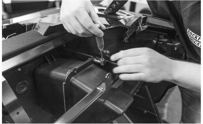
Once the glove box door is removed, remove the bolts holding the glove box in place. There are two above the chassis dash bar.
