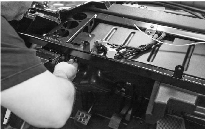
Once all of the hardware is in place, tighten all of the brackets down to the enclosure first, then to the chassis.
