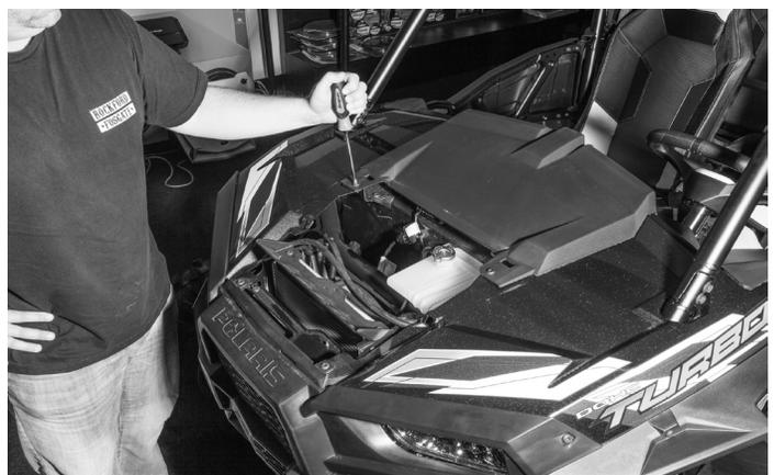
Using your hands, pull the top dash piece toward the interior of the vehicle to release it from the dash.
