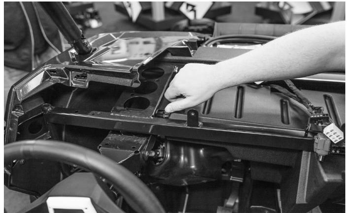
Line up the brackets with the mounting holes and insert supplied hardware into the enclosure's mounting holes. Keep everything hand tight until you get all of the hardware in place.
