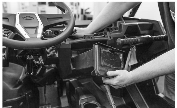
After the brace is disconnected from the center pocket, pull the pocket out of the dash.
