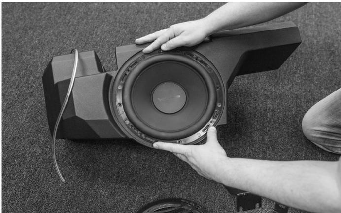
Place the subwoofer into the enclosure and line up the predrilled holes in the enclosure with the subwoofer's mounting holes.
