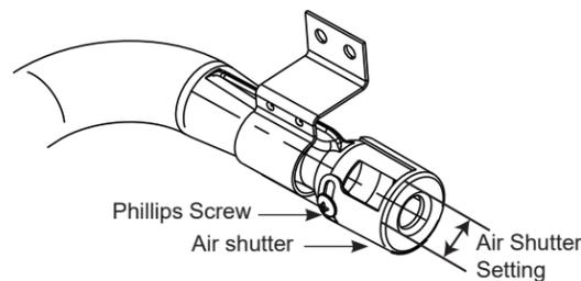
With a Phillips head screwdriver, loosen the screws securing the air shutters on the burners and adjust the air shutters according to chart above.
