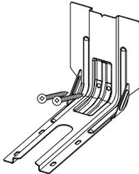
5. Using the two #10 x 1 5/8" (4.1 cm) Phillips-head screws provided, mount anti-tip bracket to the wall or floor.
