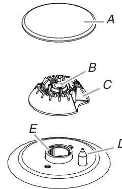
A. Burner cap      D. Igniter electrode
