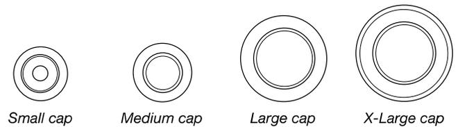
Burner caps should be level when properly positioned. If burner caps are not properly positioned, surface burners will not light. The burner cap should not rock or wobble when properly aligned.
