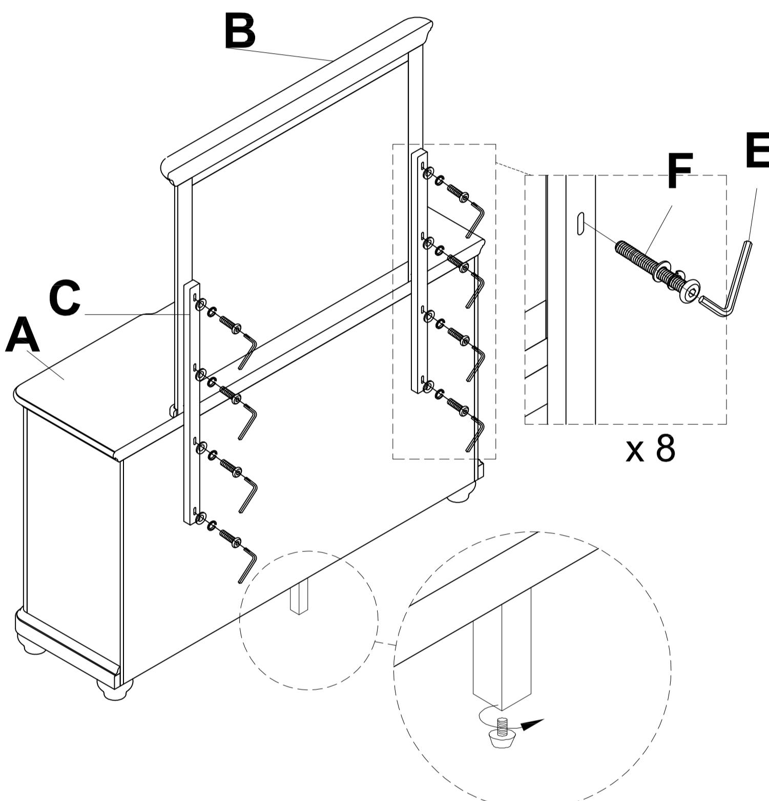
NOTE, WAIT TO TIGHTEN ALL COMPONENTS COMPLETELY UNTIL UNIT IS FULLY ASSEMBLED. THIS WILL ALLOW FOR EASIER ASSEMBLY.
