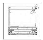
8. Move the bottom hinge hole covers from left side to right side.
