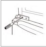
12. Place the upper door back on. Ensure the door is aligned horizontally and vertically so that the seal transfer it to the left property position. Make the middle hinge pin in the upper hole of the lower door, then tight the bolts.
