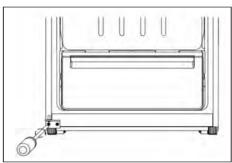
11. Make the middle hinge reverse the direction 180°, then transfer it to the left property position. Make the middle hinge pin in the upper hole of the lower door, then tight the bolts.
