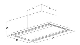
FALSE CEILING CUT:  $21^{15}/_{16}$ " x  $38^{1}/_{2}$ " \*Can be installed up to 10 ft.
