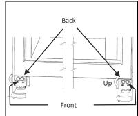
Important: Do not use a power drill and do not over-tighten the leveling bolts. Level the refrigerator to the floor, not the surrounding cabinetry, as this could affect door closing. When the refrigerator is properly leveled, door and drawer adjustment are less likely to be necessary.
