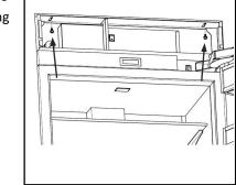
Install anchor bracket on back wall of the enclosure. The notch in the back of the bracket should be centered in the enclosure (from side to side). Secure the anchor bracket with at least two screws spaced far apart, close to the sides of the bracket. Screws must be securely threaded into wood or metal studs that are structurally sound and part of the building structure.
