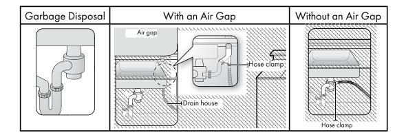
3. Check the size of the sink's drain hose connector. If needed, cut the drain hose so its end fits onto the sink connector (5/8", 3/4", or 1" as shown below). If the end of the drain hose does not fit onto the drain hose connector of the sink, use an adapter (not provided), available at any plumbing or hardware retailer.
