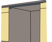
Steam protection foil must be applied where the steam escapes when door is first opened. Failure to install the steam protection foil during installation can lead to damage to the cabinets and countertop.
