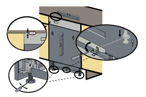
If height of the enclosure is 32 1/8" (816 mm) to 34 1/8" (867 mm), use the short leg supports as shown in the figure above.
