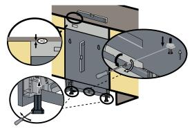
Using a level, be sure to check the dishwasher is level front to back and square to the floor and countertop.
