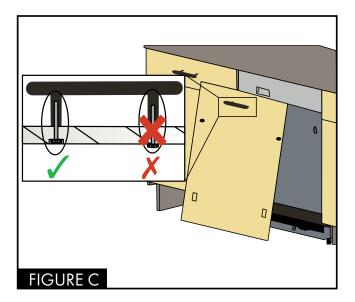
6. The upper section of the outer panel can be secured by the two mount screws (k) fastened in step 3 by sliding the panel upward after aligning those screws with the corresponding keyholes on the dishwasher door, shown with the orange arrows in Figure D. Slide the panel upward until the top edge is flush with the top of the dishwasher control panel. Once secure, the panel can swing closed, shown with the yellow arrow in Figure D.
