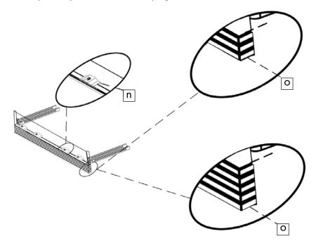
The metal back plate and adjustable plinth panel should be assembled with the kick plate brackets mounted as shown in the diagram below.
