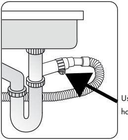
Use hose clamp for drain hose assembly to the sink.
