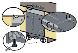
If the height is above  $34 \frac{1}{8}$ " (867 mm), use the long leg supports as shown in the figure above.
