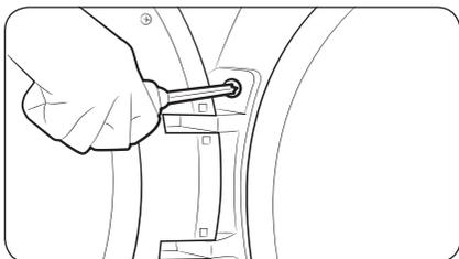
11. Place the door on the other side, and then reattach it to the dryer.
