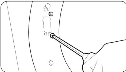
8. Re-insert the two screws that held the lever holder into the same screw holes, and then tighten.
