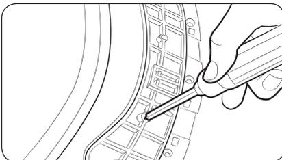
9. Remove the single screw from the back of the door hinge.
