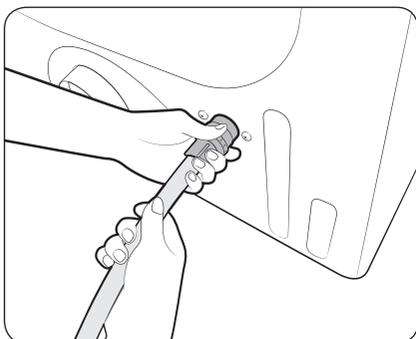
4. Connect the angled end of the water hose to the filling valve at the bottom rear of the dryer. Turn the coupling by hand until it is tight.
