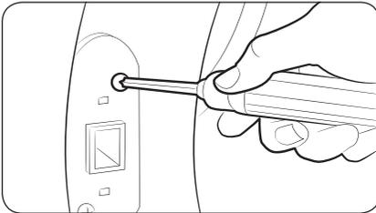
7. Remove the two screws that hold the lever holder in place, and then remove the lever holder.
