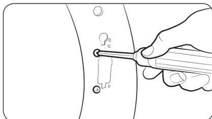
5. Remove the two screws that are above and below the cut-out in the frame front.
