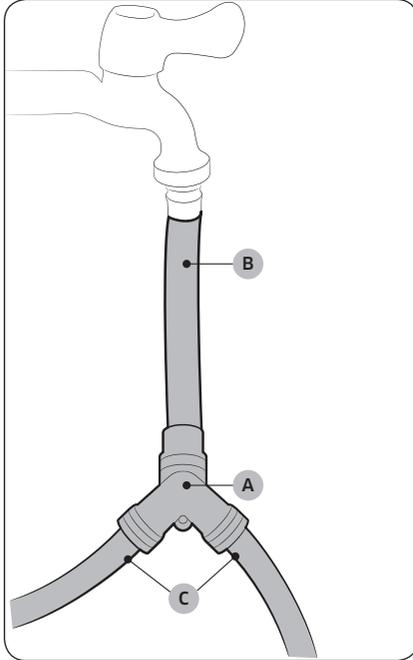
1. Close the cold water tap. If you have a washer's cold water hose attached to the cold water tap, unscrew and remove the hose. Then, connect the **short hose (B)** to the cold water tap. Turn the coupling by hand until it is tight.
