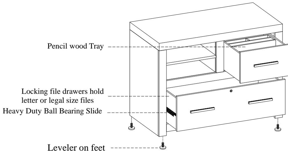
Adjust the leveler when necessary
