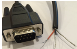
KD-3.5MDB96 after stripping wire
