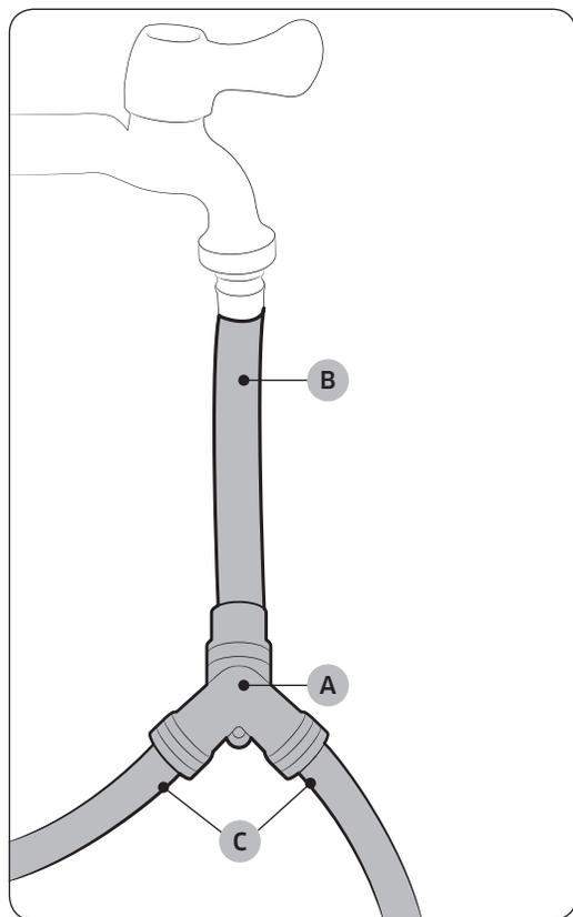
1. Close the cold water tap. If you have a washer's cold water hose attached to the cold water tap, unscrew and remove the hose. Then, connect the **short hose (B)** to the cold water tap. Turn the coupling manually until it is tight.
