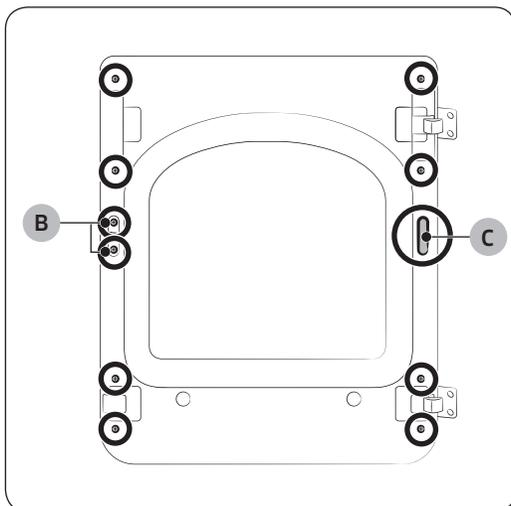
9. Remove the **hole cover (C)**, and then insert and tighten the glass holder using the removed 10 screws.
