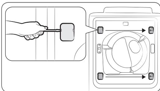
To reverse the direction of the door, we recommend that you contact a qualified technician. It is recommended to put a soft rug on the floor to prevent scratches on the door.
