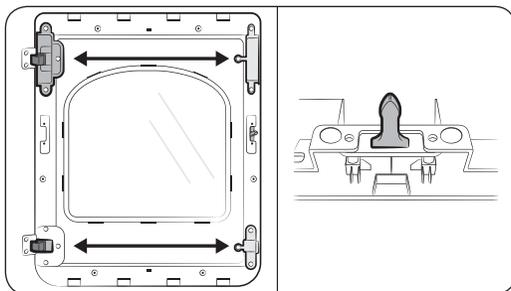
7. Remove the glass holder, and switch the positions of:
