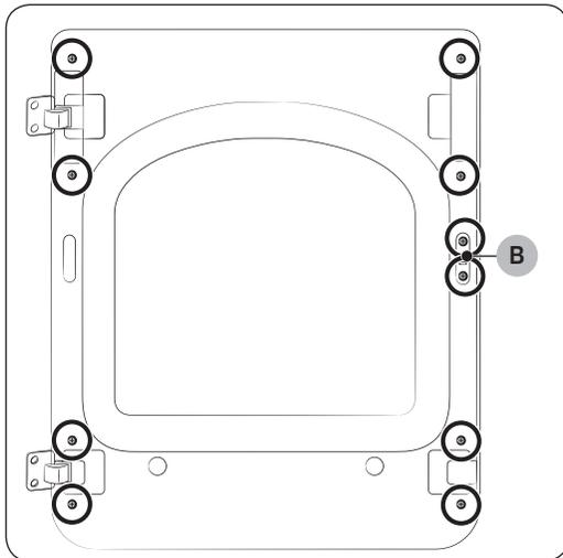
6. Locate and remove the 10 screws as shown. Note that **screw B (x2)** is longer than the others.
