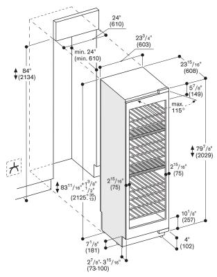
The door face dimensions are designed for a maximum gap of 1/s" (3 mm). See more details on page 252.
