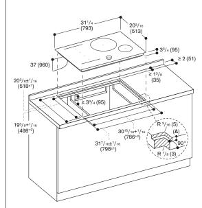
Minimum countertop thickness 13/16" (30 mm) for flush installation
