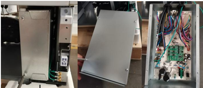
Control board epair from the lower right of the front
