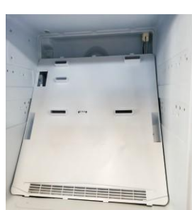
3. Remove the air duct cover
