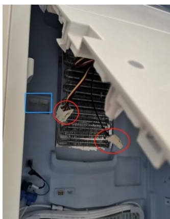
2. Unplug the terminal block
