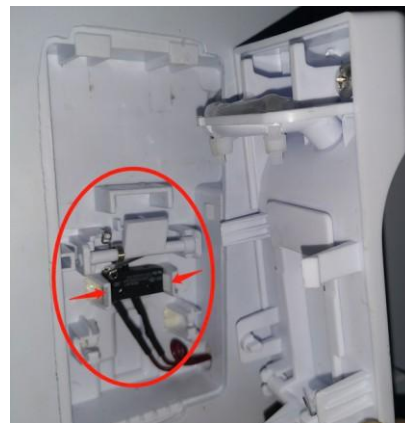
3. Carefully remove the microswitch
