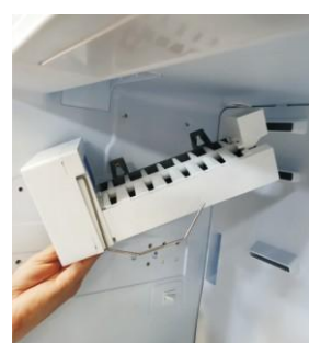
4. Unplug the terminals and remove the ice machine
