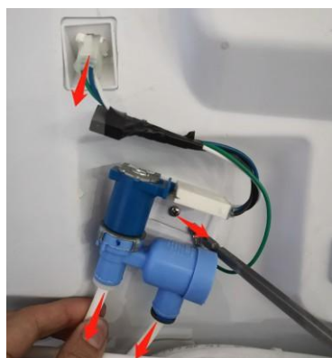
1. Remove the fixing screws and water pipes
