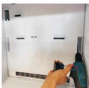
2. Remove the air duct fixing screws
