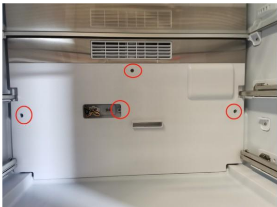
1. Remove the cover plate fixing screws
