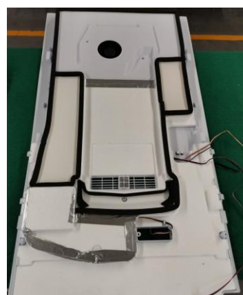
3. Remove the air duct coverplate
