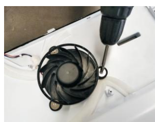
7. Removing the freezing fan
