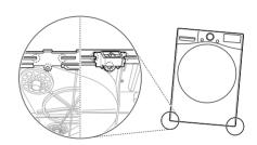
Secure the support to the dryer with a screw. Repeat steps 1 and 2 to attach the other supports, two on each side.
