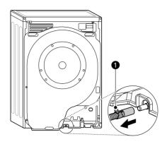
**2** Connect the drain hose of the dryer and secure the hose clamp.
