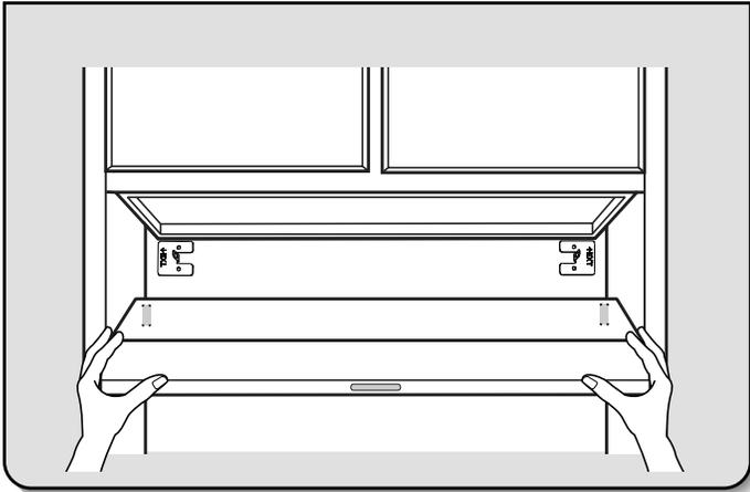
Lift the range hood into place and insert the mounting bracket tabs through the slots in the back of the range hood.
