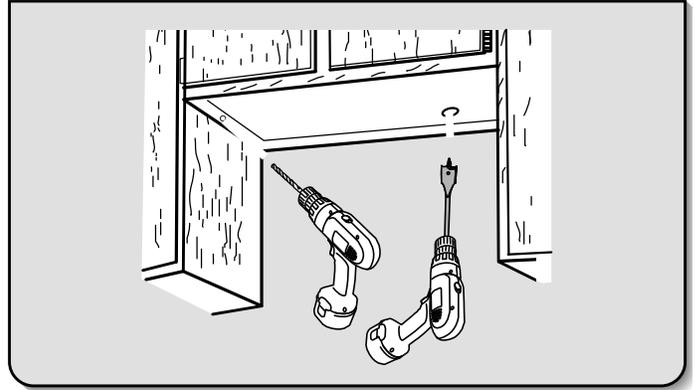
Using a 1/4" (3 cm) drill bit, drill the hole in the dot marked previously at the electrical strain relief.
