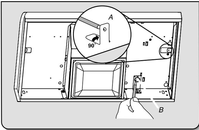
Hold the range hood firmly in place with one hand and bend each mounting tab (A) upward approximately 90°.
