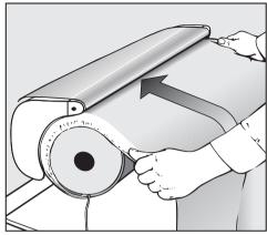
■ Press the foot pedal and "iron" the new cloth around.
