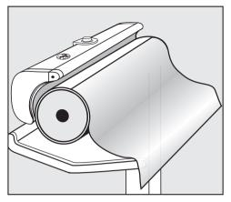
Completely unwind the padding cover attached to the roller and let it hang down smoothly.
