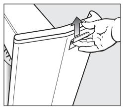
■ Hold the ironing table and release the catch, located on the right hand side at the back, underneath the ironing table.
