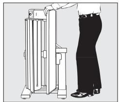
■ Hold the rotary iron with the ironing table and push or pull to move it.
