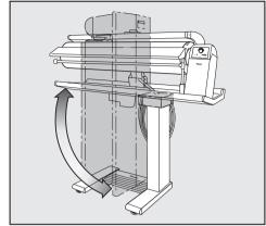
■ Swing the top section of the rotary iron to the side until it clicks horizontally into position.
