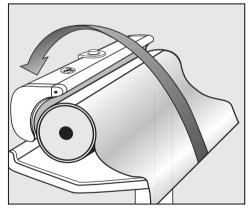
Hold the corners of the padding cover, pull taut and keeping taut lay over the heater plate.
