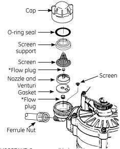
**IMPORTANT:** Be sure small holes in the gasket are centered directly over the small holes in the nozzle and venturi housing.
