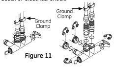
• Secure ground clamp to metal pipes.
