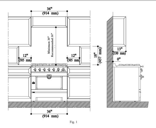
To eliminate the risk of burns or fire by reaching over heated surface units, cabinet storage space located above the surface units should be avoided.
