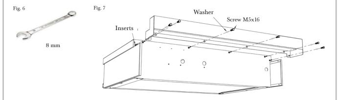
The backsplash (flue grille) is packed separately (Fig. 7). Use the screws and nuts supplied to fix the backsplash in place using an 8 mm wrench (not supplied) - Fig. 6.
