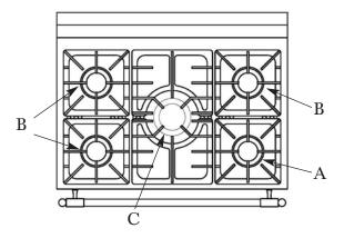
The design below shows the location of the orifice for the open top gas burners.
