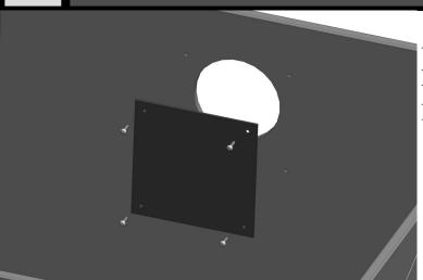
Attach Control Panel to inside of Fire Table Panel. Use (4) 1/2" Pan Head Screws.
