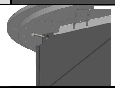
Drop Top onto Base and Secure using (4) 50mm Lags. Plug holes with 5/8" taps®.
