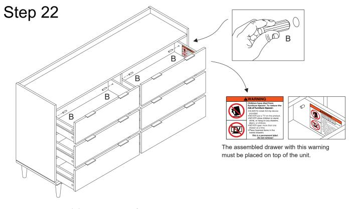
Insert wood dowel (B) on the inside of all drawers, with the drawer inside the unit, after having passed the wood dowel that is in the drawer slide.
