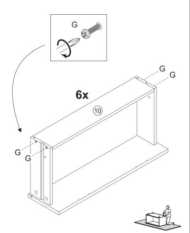
Insert part 9 and 10 between parts 5, 6 and 7. Secure part 10 with screw (G) and phillips screwdriver.
