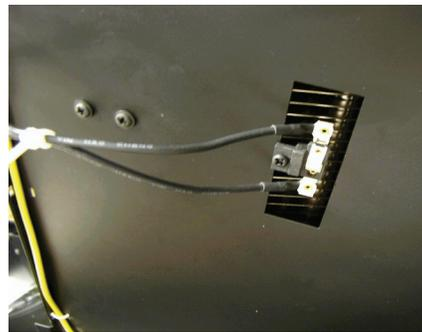
**Interior Bottom View of Voltage Selector Switch and Over Temperature Light**
