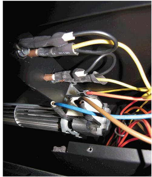
**Elements, Blower and Voltage Selector Connections**
