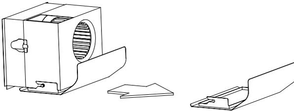
E-Z Clean blower shields are easily removed for cleaning by pulling the E-Z Clean blower shield(s) toward the front of the hood being careful to keep the tray level if the hood has been recently used.
