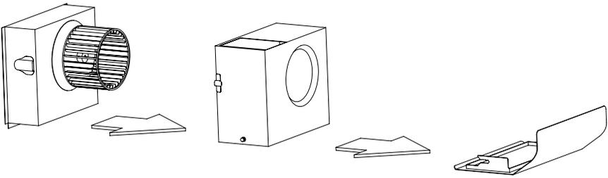
To remove the blower housing(s) and damper(s), first remove the E-Z Clean blower shield. The blower housing is removed for cleaning by unsnapping the suitcase latches (one on each side of the housing). Then, pull the housing forward and gently “tip” it downward to clear the blower wheel(s). The blower wheel(s) can be removed (if necessary) by using a 1/8" hex wrench. See part C of this section for details on how to clean the blower wheel(s).
