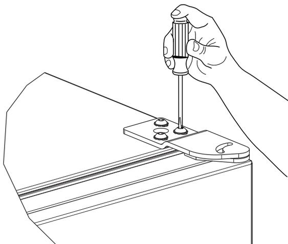
2. Remove corresponding screws on opposite side of cabinet. On some models there may be a nut behind one or both screws on either side.
