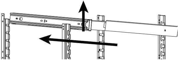
2. Tilt frame back to horizontal and line up 2 back pins with rear rail support. Line up left side of frame with rear and front rail support. Continue inserting frame until both pins engage. The front will set down slightly and lock into place. Repeat on right side.
