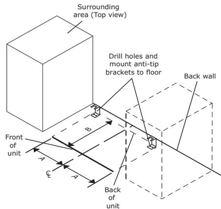
6. Use a  $\frac{1}{8}$ " drill to make two starter holes and fasten the anti-tip brackets to the floor using the screws provided.
