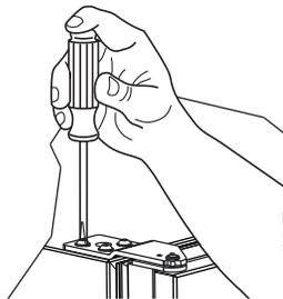
2. Rotate the door 180° and lift the door on to the bottom hinge.
