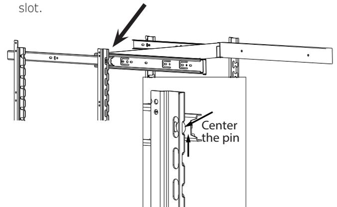
3. Pull frame towards you until all pins are clear of the slots. If only repositioning the frame, do not remove completely - go to "Storage Bin Installation" Step 2.
