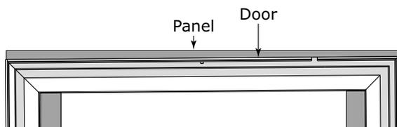
9. With panel aligned to the door, secure panel to door using clamps. A robust tape may also be used. U-Line recommends the use of bar clamps to secure the panel to the door. If using tape, be certain the tape will not damage panel finish upon removal.
