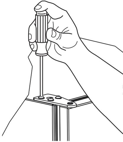
2. Rotate door 180° and set on bottom hinge.
