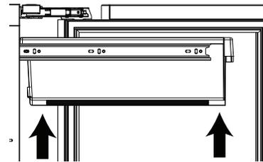
2. Firmly grasp both sides of storage bin frame and lift front end slightly (about 1/4") to center the pin in the slot.
