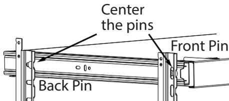
3. Fully extend frame, position bin over frame and lower (rear first) into position.
