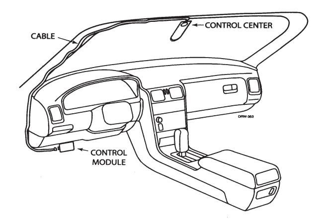
Once this control center has been installed, it must be paired with the system. Use the following procedure to first prepare the vehicle system to be paired with your remote control, then, locate your remote control type (LCD or LE/Companion) and follow the corresponding procedure. For more specific programming instructions, please refer to the programming instructions in your system's owner's guide.
