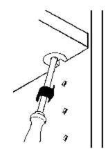
Position the screwdriver at a 25° angle.
