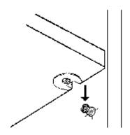
4. Using a Phillips Screwdriver at a 25° angle, tighten the Cam about a half turn.
