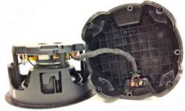
4. With the white arrows aligned, place the Acoustic Back Can atop the speaker. It should interlock perfectly with the speaker.
