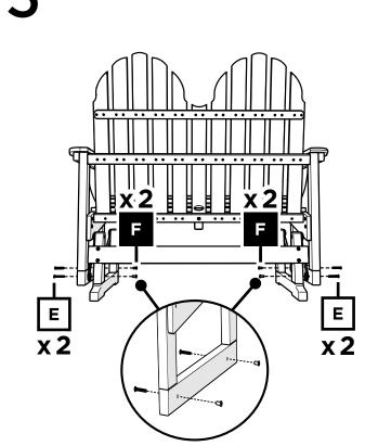
Note: Installing the base backwards could result in the glider tipping over unexpectedly.
