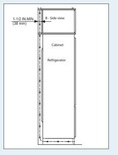
This is a built-in refrigerator-freezer with either custom finished door panels or stainless steel doors. The unit is not intended for freestanding use and has to be installed inside a cabinet. This type of cabinet must be carefully constructed using the proper dimensions and it must provide proper ventilation to ensure proper appliance operation.
