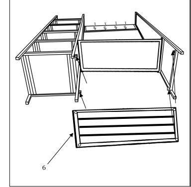
STEP# 8: Tighten the bolts to lock the iron shelf(6) as shown below.
