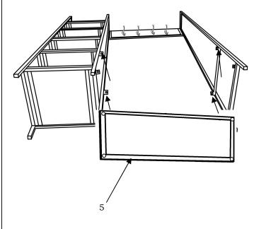
STEP# 6: Tighten the bolts to lock the wooden shelf(5) as shown below.
