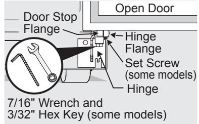
5. Reinstall the set screw, locking the door height.
