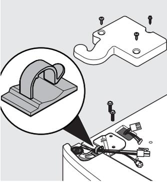
3. Release the wires from the routing clip.
