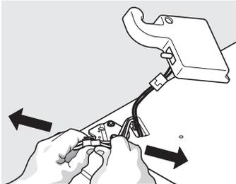
Disconnect the multi-wire cable connector located above the top hinge. Press the cable and lock and separate the 2 cables.
