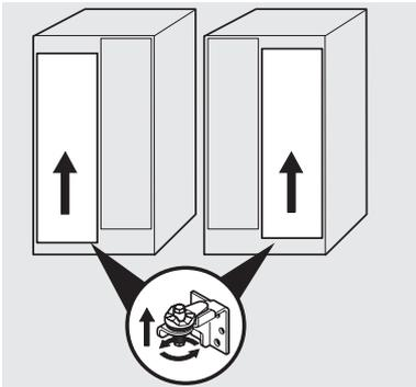
4. After leveling, verify the door stop contacts the lower hinge and the top of the door does not contact the upper hinge through full movement of the door (from fully closed to fully open).
