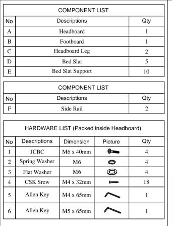
ASSEMBLY TIPS 1.Take Out hardware from box and sort by size. 2.Please check to see that all hardware and parts are present prior start of assembly. 3.Please follow attached instructions in the same sequence as numbered to assure fast and easy assembly
