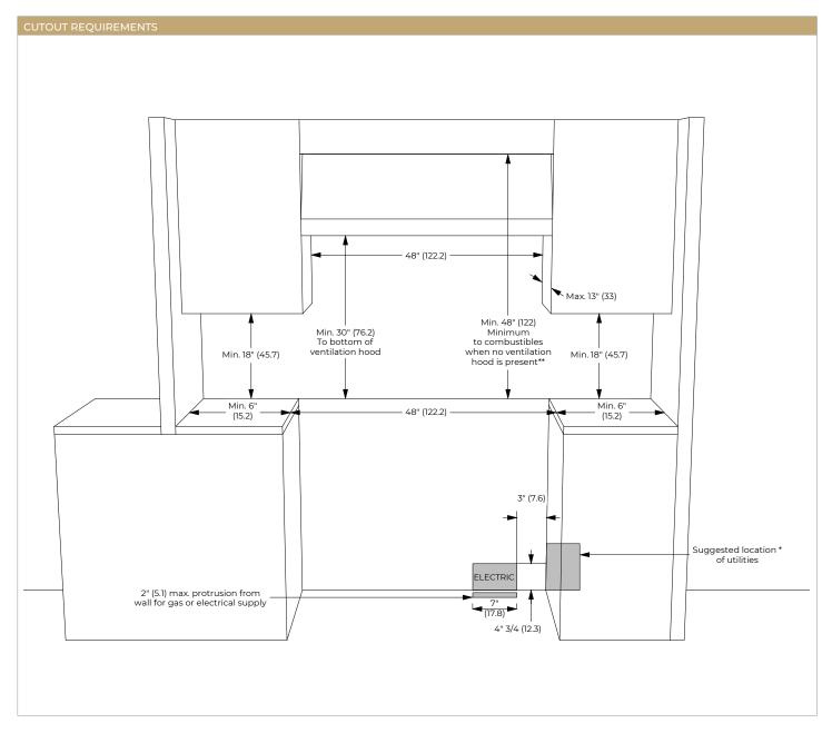
\*\*NOTE: Ensure your installation also complies with local and national building and fire codes. If the surface of the entire back wall above the range and below the hood is not composed of a non-combustible material then the 9" accessory back guard must be used. \*Consult local code for exact location requirements.
