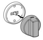
To remove the knob ring, turn it counterclockwise to release the tabs on the knob ring from the notches.
