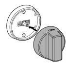
**5** Push the knob onto the shaft as far as possible so it fits snugly.
