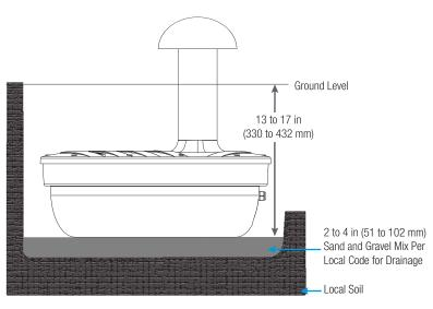
**NOTE:** The hole must be deep enough to allow a 2 to 4 in (51 to 102 mm) layer of drainage material (sand and gravel mix or other material approved by local codes) and position the base of the speaker 13 to 17 in (330 to 432 mm) below ground level.
