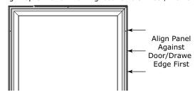
Due to differences in floor construction or surrounding cabinetry, the panel may not sit flush with the top of the door/drawer.
