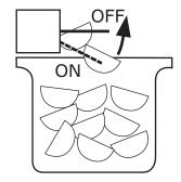
**To turn off ice production:** Raise the bin arm into an upright and locked position. The unit will preserve temperature for ice storage.
