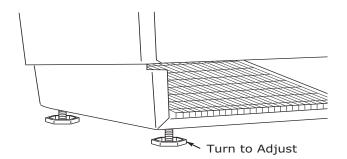
3. Confirm the unit is level after each adjustment and repeat the previous steps until the unit is level.
