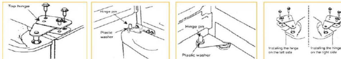
If you notice the door not hanging straight, loosen the top hinge screws, adjust the door until it is level and tighten the screws.
